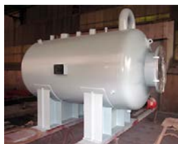
Thermal power plant water tank D:3m L:5m, Capacity: 13 m 3
