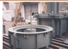
Shielded container for Nuclear power generation Interior: cast lead
